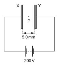
A small oil drop at P carries one excess electron.
